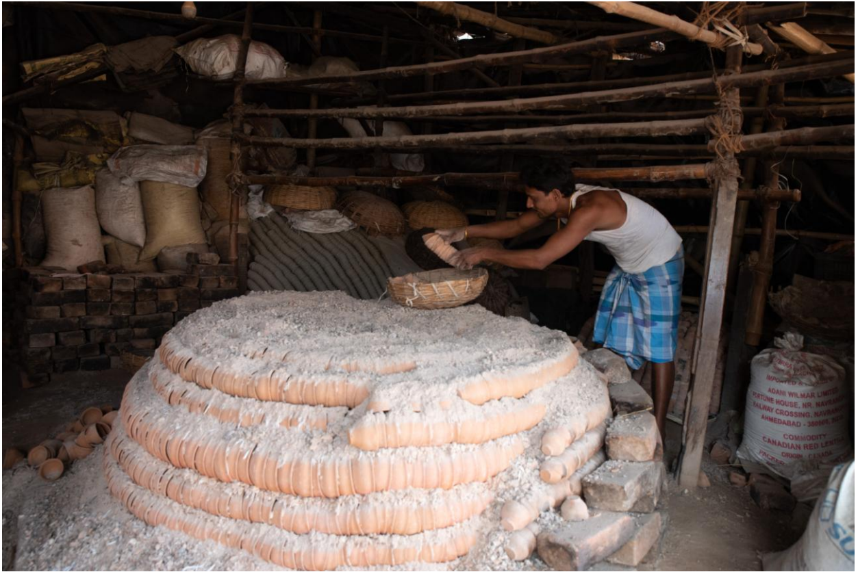
Plate 39 – Bhar making in the handmade Vati ( furnace)
